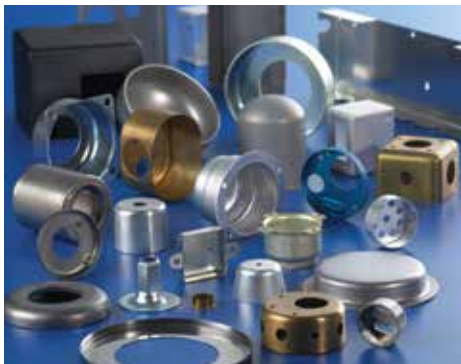
Draws up to 3" deep and 8" in diameter
