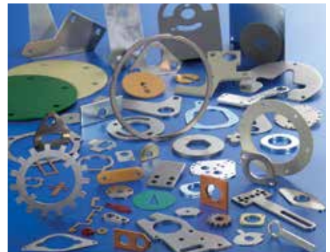
Flat blanking and piercings up to 12" by 12"
