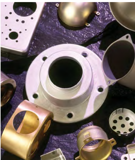
Draws up to 3" deep and 8" in diameter
