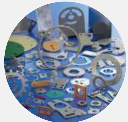
Flat blanking and piercing up to 12" by 12"
